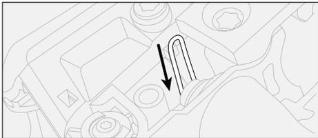
Carefully push the brake lever cover with the MAGURA logo onto the brake lever.
